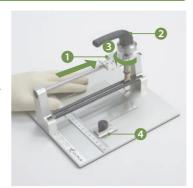
For precisely determining the cutting position, use of magnetic substrate guide **4** (sold separately) is recommended.
